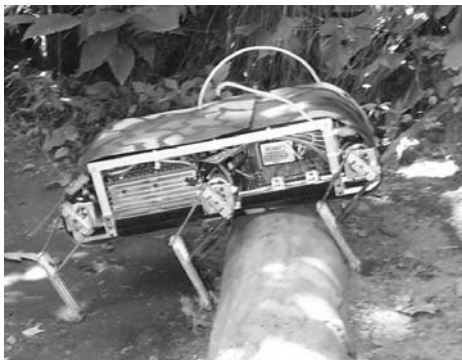
Figure 3 RHex, a six-legged walking (left) and running (right) robot with compliant legs
