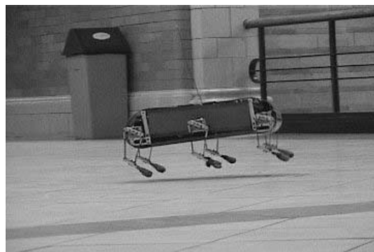
Figure 3 RHex, a six-legged walking (left) and running (right) robot with compliant legs
