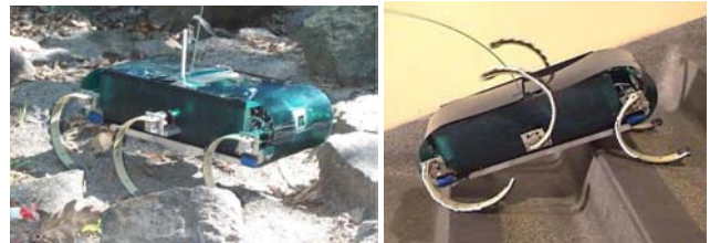
Figure 8: RHex in rough terrain and on stairs.
