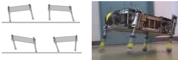
Figure 6: Illustration of a bounding gait (left) and Scout II bounding (right).
